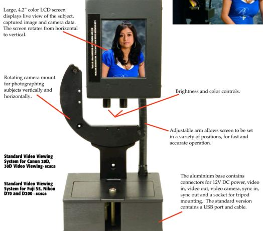
An optional USB port and Software allow the live and captured images to be viewed on a PC. The live image window can be open and viewed, even when an image and data management application or other programs are being used.
